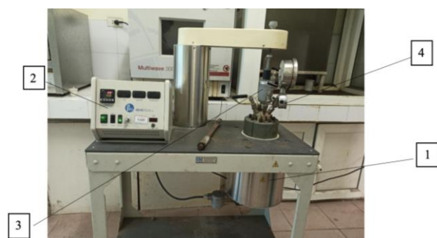
Fig. 4. Autoclave apparatus: 1 – furnace, 2 – control system, 3 – mixer, 4 – furnace lid with pressure meter
