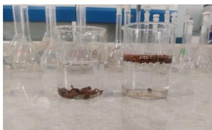
Fig. 3. Scoria hydrophobic property before and after modification
