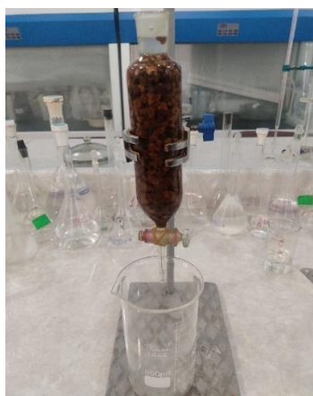
Fig. 8. Mini-filter in the form of separatory funnel
