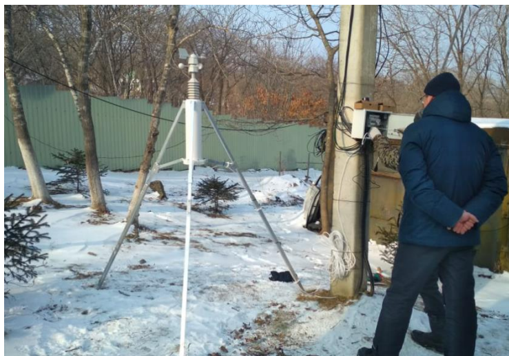
Fig. 2. Automatic monitoring station for the measurement of ambient air parameters, deployed at point 1 M
