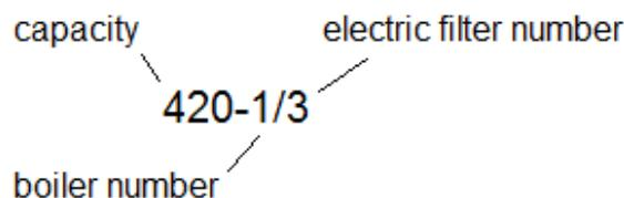
Fig. 1. Designation of samples from different boiler and electric filters fields
