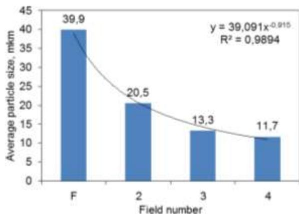
**Fig. 5.** Reduction in the size of the ash particles of electric filters with an increase in the field number
