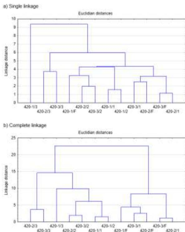
**Fig. 3.** Dendrogram of hierarchical clustering according to the NRN specific activity in the ashes captured by various fields of the UG3-3 type electrofilters: a) clustering by single linkage method; b) clustering by complete linkage method
